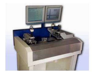
The SBS420 is an unique machine designed scribing & breaking & sorting delicate component, such borosilicate lid
