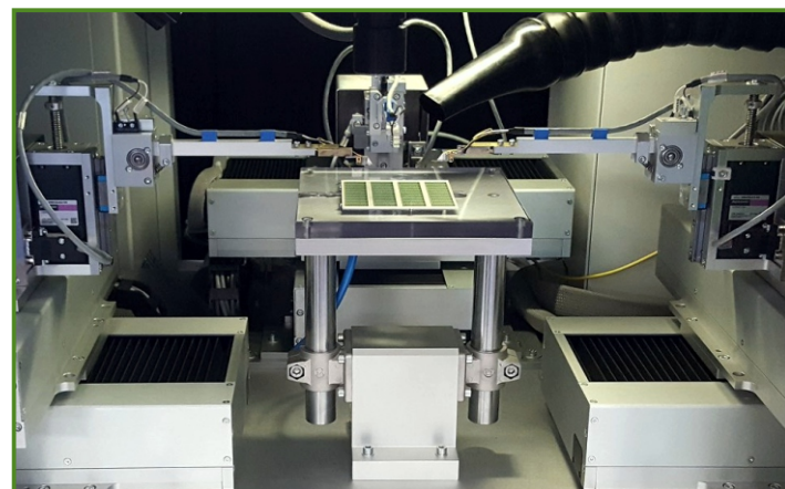
EXAMPLE OF PROBING SYSTEM WITH 3 FLYING PROBES (WITH ACTIVE PIN GUARD MODE)
